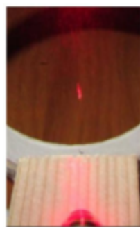
Photo of Laser light bending across a human hair that acts as the central post in the double slit experiment.
